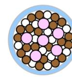
Spray-mist grows together with micro-air and clay in the process of cohesion. And then, polymer make the surface surrounding, it come to float to water-surface by the pretension density is light.
